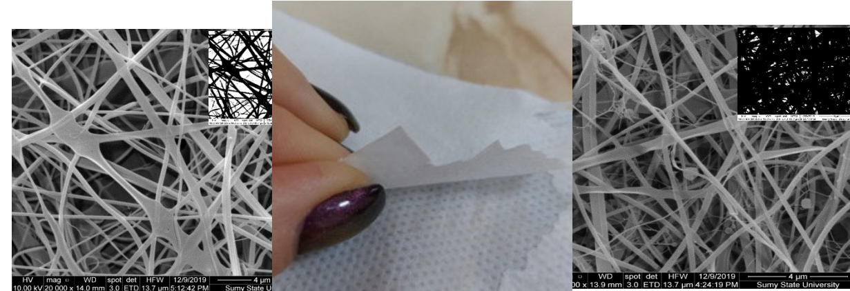
Figure PLA polymer membrane with high porosity
